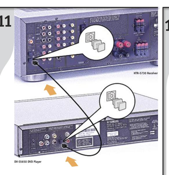
**DVD Player Optical Connection (optional)** Remove dust cap on optical input as shown on insets. Connect optical cable (not included) to receiver. Connect optical cable to DVD player from receiver.
