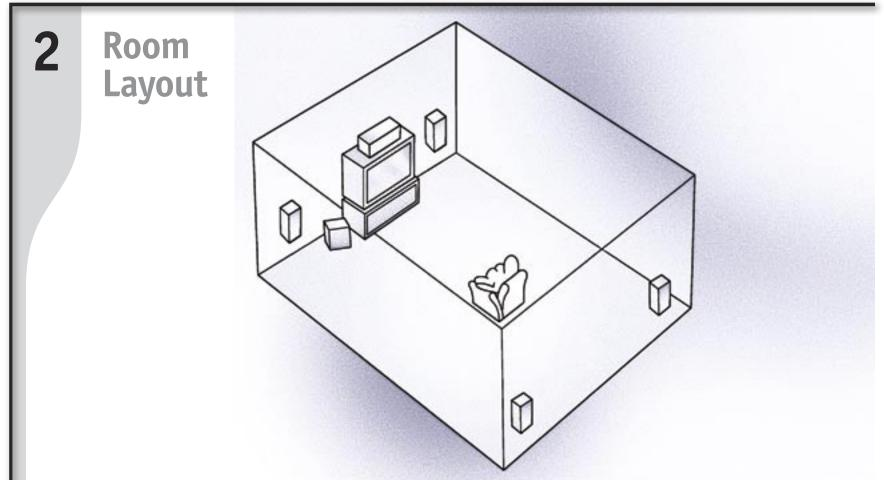
Speaker Placement After connection of the speakers place them so they appear in the approximate positions as shown in the diagram above.
