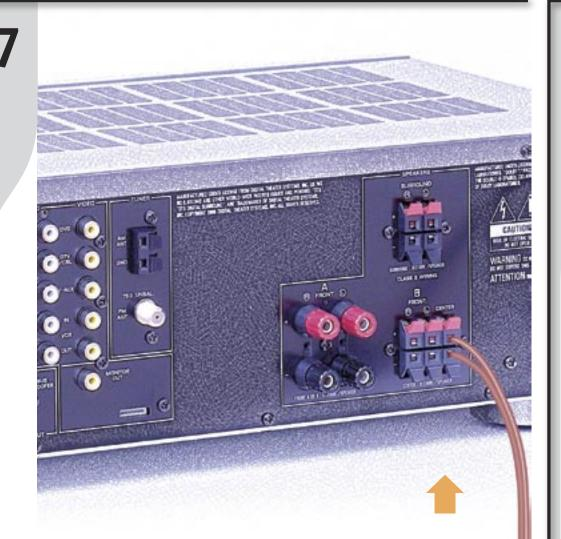
**Connect Center Speaker** Positive (+) side of the wire with white stripe attaches to (+) terminal. Negative (-) side attaches to (-) terminal. **CAUTION** Receiver must not be plugged in while connecting speakers.
